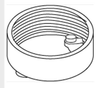
Installed either before or after concrete pour to create activation from duct. NOTE: Drill a 2 1/2" [64mm] hole in concrete and a 2 1/4" [57mm] hole in duct.
