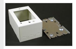
Designed especially for use in the installation of signal system and alarm wiring. Base has 1/2" trade size KOs. Larger gang boxes available by special order. Single-gang: 4 5/8" L x 2 7/8" W [117mm x 73mm]. Accepts NEMA single-gang standard faceplates. NOTE: Certified to Canadian Safety Standards for sale in Canada. When ordering these products, change the "V" color prefix to "vc" or the "WH" color suffix to "WHC" to denote the Canadian versions.
