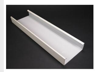
.054" [13.7mm] galvanized steel. Packed five 10' [3m] lengths per carton. Base has two 9/32" [7.1mm] diameter KOs on centers of approximately 18" [457mm] throughout. No KOs on 1 1/4" [32mm] from each end.
