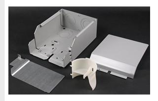
Full capacity entrance end fitting. Has concentric 3/4", 1", and 1 1/4" trade size KOs on end and bottom for feeding 4000 Series Raceway. Includes removable divider and 1 1/4" [32mm] bend radius control insert for UTP/STP and fiber cable installations.
