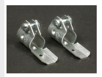
Connects 14/2, 14/3, 12/2, and 12/3 "MC" and armored cable to Wiremold fittings. A short piece of 500 or 700 Series Raceway (1 5/8" [141mm] min.) must be used between connector and Wiremold fittings. Not for use with 1/2" [12.7mm] flex conduit.
