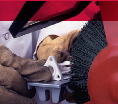
Deburring a plastic part using a nylon brush.
