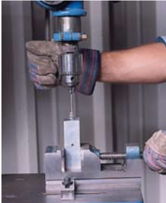
Crosshole deburring an aluminum manifold.
