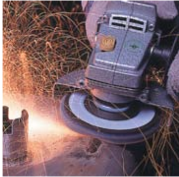
Weld blending on an automotive part.
