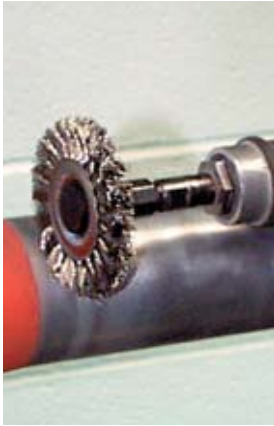
Removing rubber coating from a roller.
