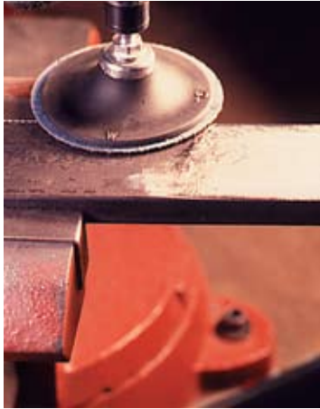
Removing mill scale on a hot rolled steel part.
