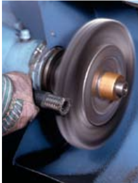
Removing rubber coating from a hydraulic hose.
