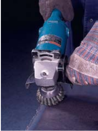
Removing slag from the edge of a flame-cut steel plate.
