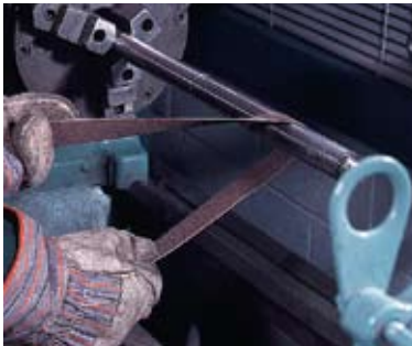
Polishing the O.D. of a part turned in a lathe.
