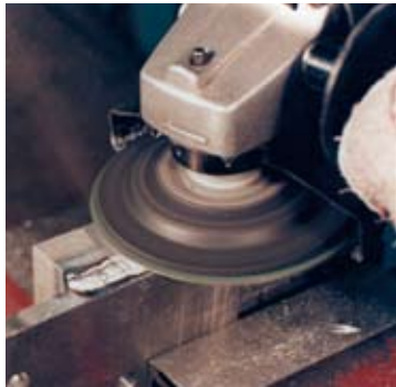
Blending aluminum welds on a machine bracket.
