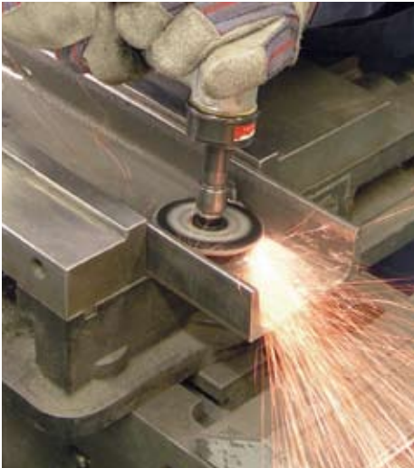
Blending excess brazing material on a machine component.
