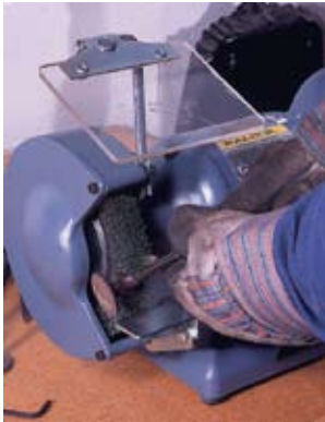
Remove carbon build-up from an automotive valve.
