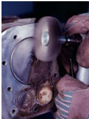
Removing carbon build-up from an engine.
