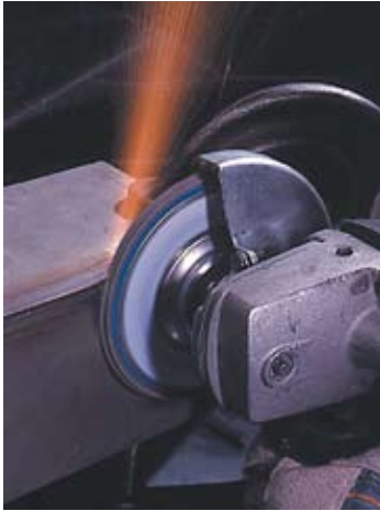
Blending a corner weld on a stainless steel cabinet.
