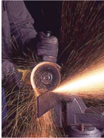
Notching a piece of steel bar prior to welding.
