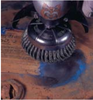
Removing rust and a label from a 55 gallon drum lid.
