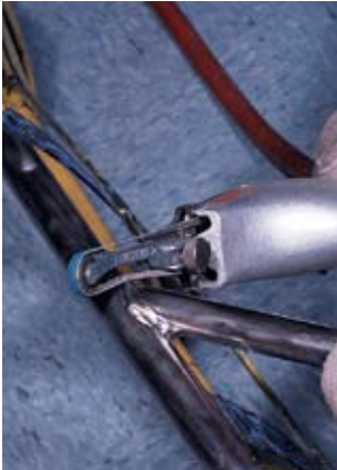
Blending a weld using a portable file belt.
