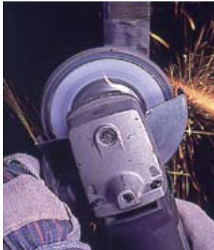
Blending and finishing edges of a flame-cut steel part.
