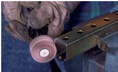
Deburring perforated steel channel after saw-cut.
