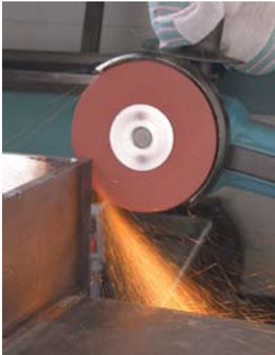
Grinding welds on a fabricated steel part.
