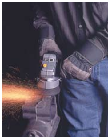
Removing gates and risers from an iron casting.
