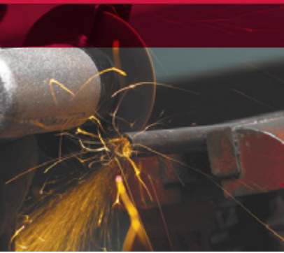
Cutting a piece of Steel tubing to length.
