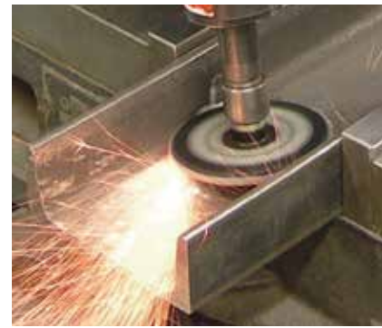
Blending welds on a steel rule die with a BobCat disc.
