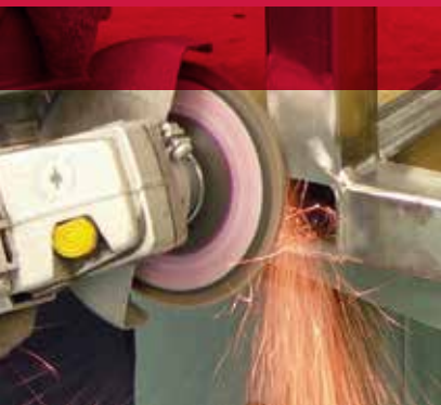
Grinding welds on a fabricated Steel part.
