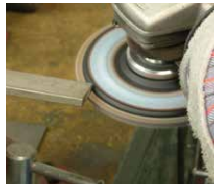
To trim backing, run against a sharp edge until desired backing diameter is achieved.
