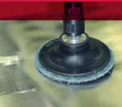
Finishing the surface for a stainless steel part for the food service industry.
