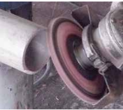
Grinding and beveling Stainless Steel tubing with a Saber Tooth abrasive flap disc.
