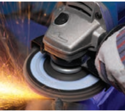
Blending and finishing a weld.
