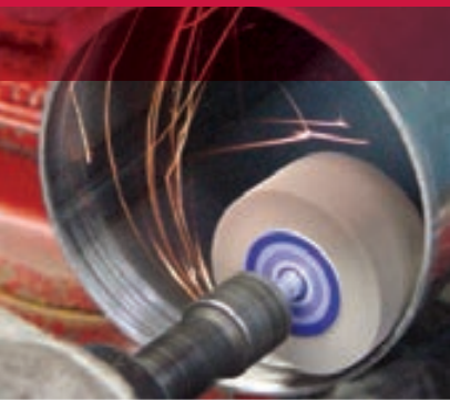
Removing burrs from the inside diameter of a cut tube.
