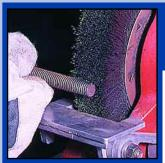
Cleaning threads with a crimped wheel brush.
