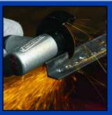
Cutting a piece of angle iron to size with a cut-off wheel.
