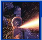
Notching a steel bar prior to
