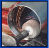
Removing burrs from the inside diameter of a cut tube.
