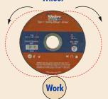
**Counter rotation of the work-piece** is recommended for cutting large cross sections (over 8") and when cutting tubular stock.
