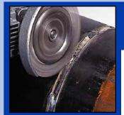
Cleaning a weld with a knot wire wheel brush.
