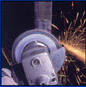
Blending and finishing edges of a flame-cut steel part.
