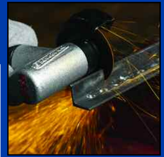
Cutting a piece of angle iron to size with a cut-off wheel.
