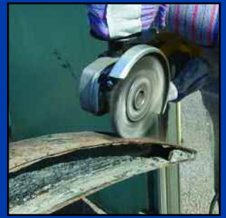
Prepping a machine guard for on-site welding and repair.
