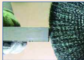
Correct Wire Tips Doing the Work
