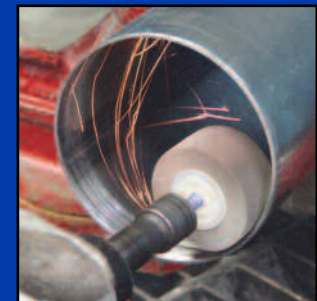
Removing burrs from the inside diameter of a cut tube.
