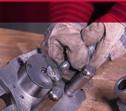
Removing galled spots from a metal forming die.
