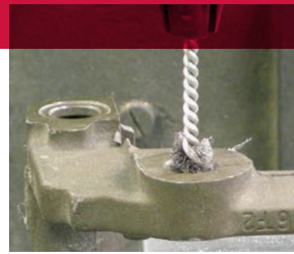
Removing zinc coating from holes in a brake bracket.
