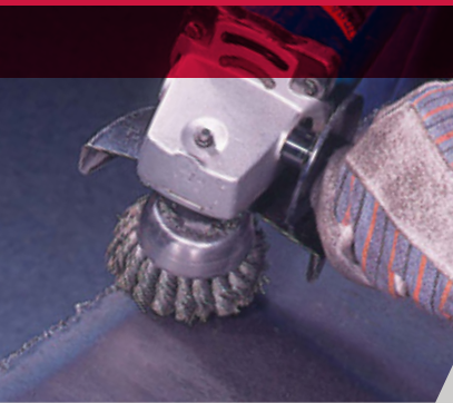
Removing slag from a flame-cut Steel plate.
