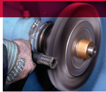
Removing rubber coating from a hydraulic hose.
