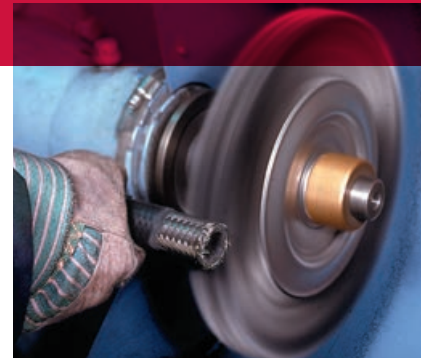
Removing rubber coating from a hydraulic hose.
