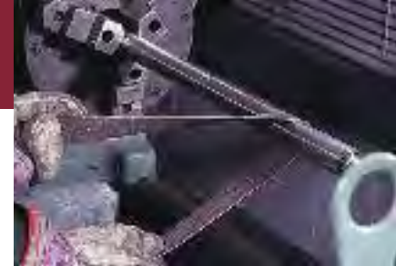
Polishing the O.D. of a part turning in a lathe.
