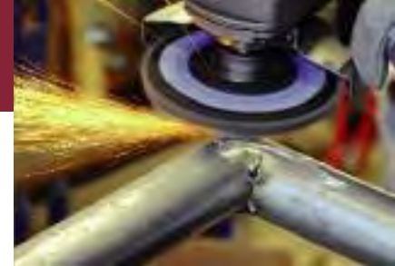
Weld blending on the corner of a security gate with a Tiger Paw XHD.
