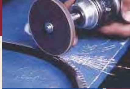
A unitized wheel deburring a ring gear.
