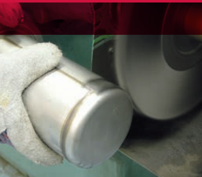
Removing heat discoloration from a stainless steel canister.
