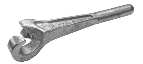
TITAN "100 SERIES" VALVE WHEEL WRENCHES are made from aluminum-magnesium to reduce the chance of sparks when opening stubborn valves.
