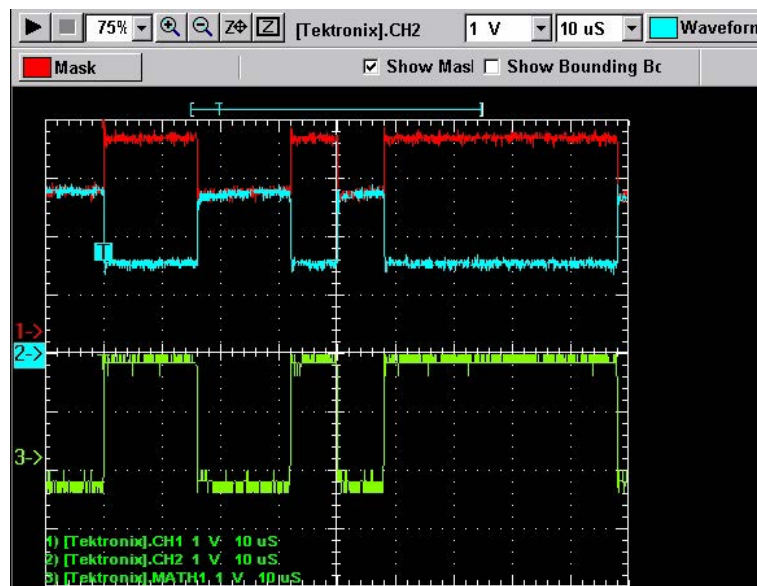
Oscilloscope capture of the differential CAN signal. The CAN high and low components are shown with the resulting difference below.
