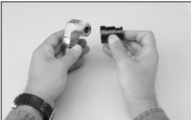
Figure B5 — O-ring Installation Using CORG Assembly Tool
