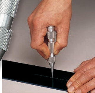
Easy one-hand precision center punching
