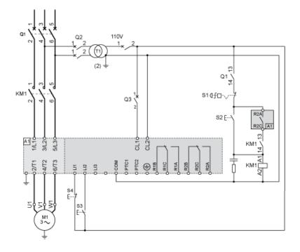
110 Vac control, Logic Inputs (LI) 110 Vac, 2-wire control, freewheelstop
