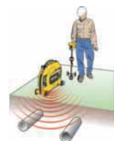
Induce a signal to locate utilities
