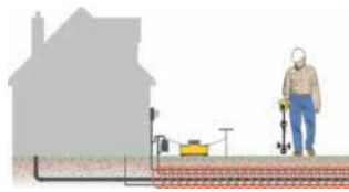
Direct connect to utility lines
