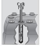
SECOND – Remove Drill Guide. Drill out the small center hole to larger diameter for receiving the "longrip" Extractor.
