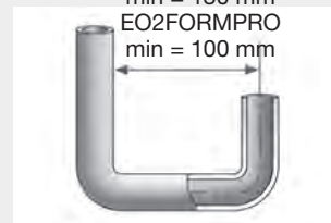
● Minimum clearance of U-shape bends
