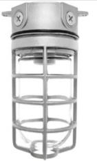
Box mount, die cast aluminum with built-in junction box and sturdy mounting lugs. Medium base socket, 1/2" or 3/4" NPS hub size and a variety of globes. incandescent lamp A21 for 100 Series, PS25 for 200 Series. Lamp not supplied.
