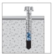
When re-used to pilot a new anchor hole, 1 or 2 additional applications or re-uses are possible. The high double lead thread should be checked for excessive wear. Base material conditions (hardness and density) will affect re-usability.
