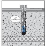
The Wedge-Bolt anchor can be installed at shallower embedment depths than traditional wedge or sleeve anchors reducing the chance of striking reinforcing bars or embedded cables. Drilling time and bit wear can be reduced resulting in significant savings.
