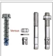
The Wedge-Bolt anchor is a onepiece unit which features a finished hex head formed with an integral washer, a patented dual lead thread, and a chamfered tip. A one-piece design eliminates the possibility of lost anchor parts or improper assembly.
