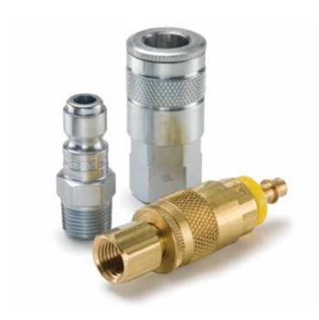
Parker's 10 Series Pneumatic Couplers are the original Tru-Flate design. 1/4" body size has a brass body, while standard 3/8" and 1/2" body sizes have all steel construction. Sleeve options include Sleeve-Lok and Grip-Ring sleeve.
