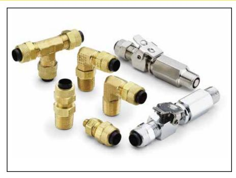
A preassembled compact compression fitting. An exclusive acetal copolymer sleeve has superior resilience to resist creeping and stress caused from compression. Poly-Tite nuts will rotate around the sleeve as it tightens to prevent twisting and weakening of the plastic tubing.
