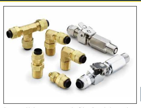
A preassembled compact compression fitting. An exclusive acetal copolymer sleeve has superior resilience to resist creeping and stress caused from compression. Poly-Tite nuts will rotate around the sleeve as it tightens to prevent twisting and weakening of the plastic tubing.
