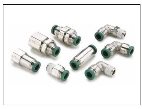
A compact one-piece push-to-connect fitting. Designed for low pressure circuits where assembly, disassembly and reassembly is important. Stainless steel grab ring grips the tubing to provide retention. Swivels are featured on all male pipe threaded shapes for installation in tight places and for precise positioning. Prestolok should not be used for live swivel applications. Prestolok fittings come with a pre-applied white acrylic sealant.
