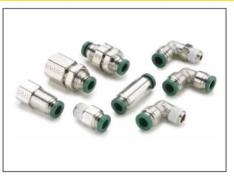
A compact one-piece push-to-connect fitting. Designed for low pressure circuits where assembly, disassembly and reassembly is important. Stainless steel grab ring grips the tubing to provide retention. Swivels are featured on all male pipe threaded shapes for installation in tight places and for precise positioning. Prestolok should not be used for live swivel applications. Prestolok fittings come with a pre-applied white acrylic sealant.
