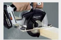
3 Eject dust to the rear of the machine
