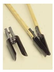
The diameter of the hole produced by each digger is approximately 6". The operating action for the solid-handle digger begins with the handle together. The handles are then pulled apart with a side-to-side motion to capture the load. With the split-handle digger, the operator uses a forward-and-back motion. The split handle design has a wider blade opening, which allows for a larger hole to be dug.
