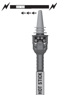
Fig. 2: Finding a cable fault
