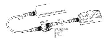
Connection of Smile 11 ROx to Orion through M12-3R. For connection to any control module compatible with OSSD outputs.
