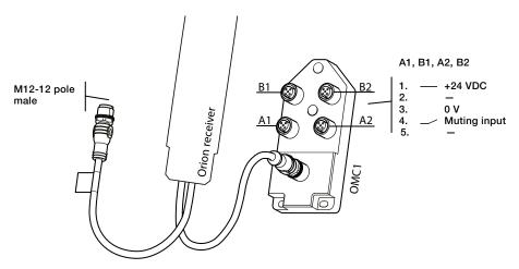
NB: Cable with M12-5 male + female connectors shall be used between muting sensors and OMC1 inputs A1, B1, A2, B2.
