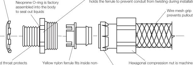
Insulated throat protects insulation on wires during pulling; yellow color easily seen by inspectors Yellow nylon ferrule fits inside nonmetallic conduit to hold the shape; barb in designed to assure liquidtight seal even with non-square cut; ferrule is keyed to fit into body to prevent conduit twisting Hexagonal compression nut is machine steel through 1" malleable iron on larger sizes; tapered interior compresses sleeve over conduit sealing out liquids and preventing pullout
