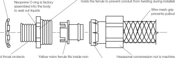
Insulated throat protects insulation on wires during pulling; yellow color easily seen by inspectors
