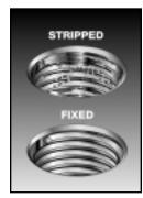
damaged thread is repaired with Heli-Coil inserts. The Heli-Coil threaded insert provides stronger, more reliable threads than the original tapped hole and at the same time eliminates the possibility of thread wear, corrosion, galling, seizing and rust.
