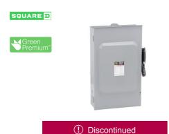
Safety switch, heavy duty, fusible, 200A, 3 wire, 2 pole, 1 neutral, 60hp, 240VAC/250VDC, NEMA 3R, bolt on hub provision
