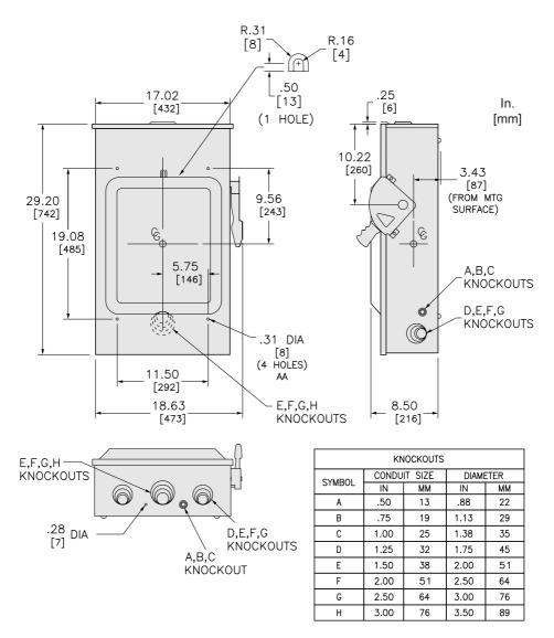
WHEN MOUNTING, ALLOW 4.00/[102] MIN. CLEARANCE BETWEEN ENCLOSURES FOR OPENING OF SIDE HINGED DOOR. TOP OF NEMA TYPE 3R DEVICES HAVE PROVISIONS FOR MAX 2.50/[64] BOLT-ON HUB.
