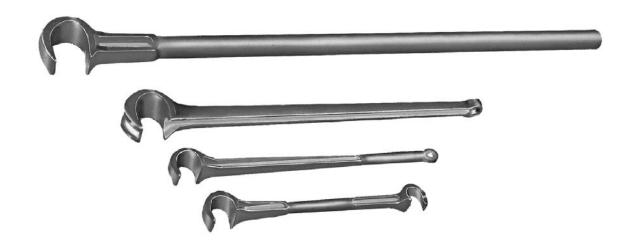
TITAN VALVE WHEEL WRENCHES are used to provide leverage on hand operated valve wheels. This series of wrenches permits a smooth snap "hammer-action" to make opening and closing stubborn valves easy. Each wrench will fit a variety of sizes and shapes of valve wheels. The special shaped opening in the wrench reduces the chance of slippage when working in overhead or crowded positions.
