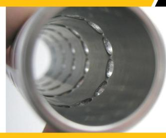
When deburring cross drilled holes using the Flex-Hone, it is helpful to first stroke and rotate the tool in a clockwise direction and then remove the tool from the bore, reverse the spindle and then stroke and rotate in a counterclockwise direction. This promotes a more symmetrical deburring pattern and prevents the burr from folding back into the cross-hole.
