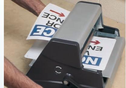
**Step 1:** Peel away the first 1 1/2" of liner from the back of PowerMark™ printer output. Apply to blank panel, aligning edge of label with edge of panel.
