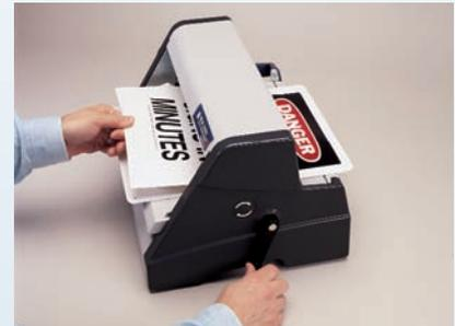
**Step 2:** Insert sign into laminator and rotate handle until first 1" of sign is "pinched".
