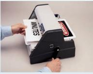
**Step 2:** Insert sign into laminator and rotate handle until first 1" of sign is "pinched". Stop. Then grasp liner of sign and pull at
