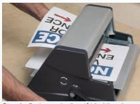
Step 1: Peel away the first 1<sup>1</sup>/2" of liner from the back of PowerMark<sup>™</sup> printer output. Apply to blank panel, aligning edge of label with edge of panel.
