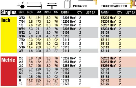
\*The 3/32, 7/64, 1/8, and 9/64 inch blades, and the 2, 2.5 and 3mm blades are straight hex blades to prevent breakage.
