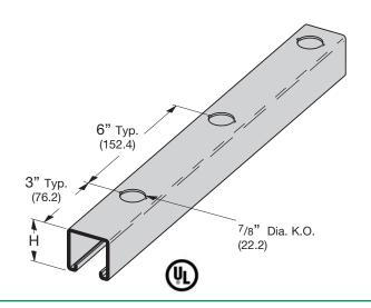
B22SHA (BACK TO BACK SH TYPE CHANNEL) • For beam loads use 90% of Channel Loading Chart
