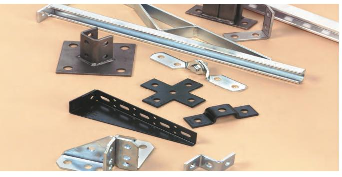
This section offers a full selection of fittings and accessories to complete our strut system. Fittings are made from hot rolled, pickled and oiled plate or strip steel in accordance with ASTM A1018 33,000 PSI min. yield, unless noted.
